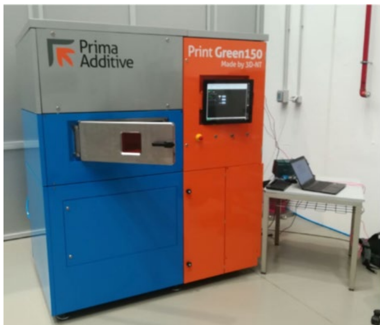
3D-NT industrial SLM system green laser source
