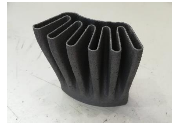
Geometry test in AISI 316L
