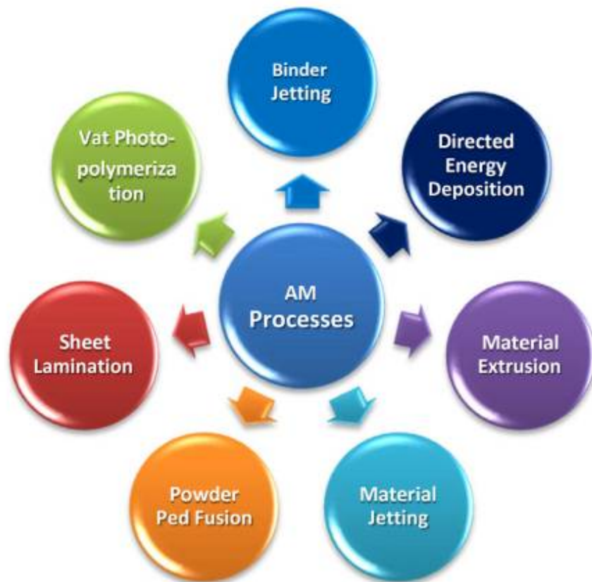
Fig. 1. Classification of AM processes based on ISO/ASTM 529000:2015.
