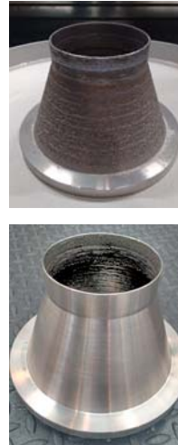
AISI 316L, P = 720W , f = 750 \text{ mm/min} , \dot{m} = 18 \text{ g/min}
