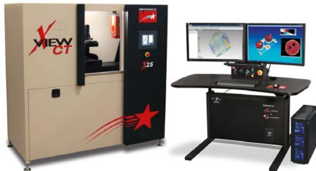
3D X-Ray CT- Scan microtomograph y ( NSI 160 kV)
