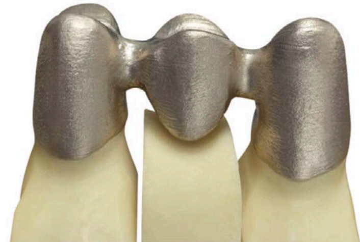
Wirobond C+ three- unit bridge manufactured by BEGO USA using their EOS additive manufacturing system. Support anatomy, precise marginal integrity and smooth surfaces are produced consistently from every STL file (Source: BEGO USA).
