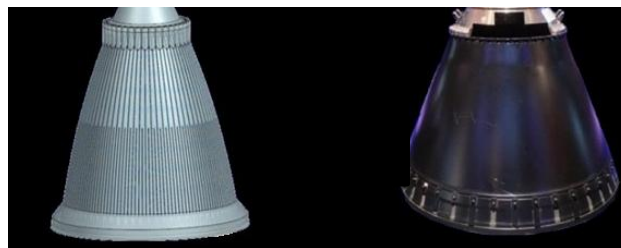
Figure 1: On the left, the design of a generic nozzle; on the right, the cryogenic engine Ariane 6, upper stage.
