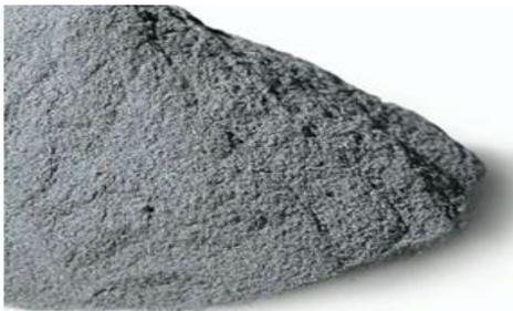
Metal powder is bound in plastic (Just like metal injection molding) and then formed into feed rods
