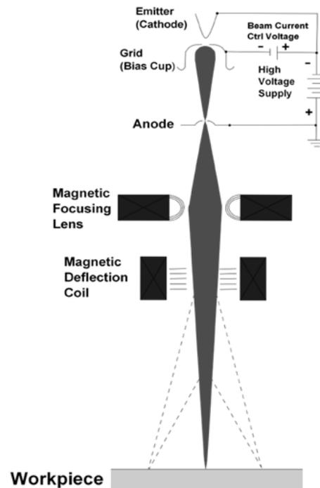
Figure 2 – schematic view of an EBM machine [6]
