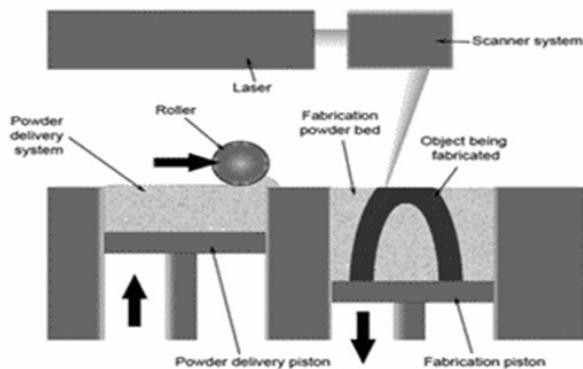
Figure 1 – schematic view of a laser based sintering/melting machines [5]
